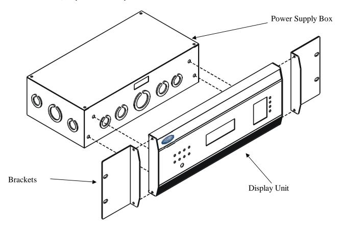
To install the Master in a 19-inch rack
